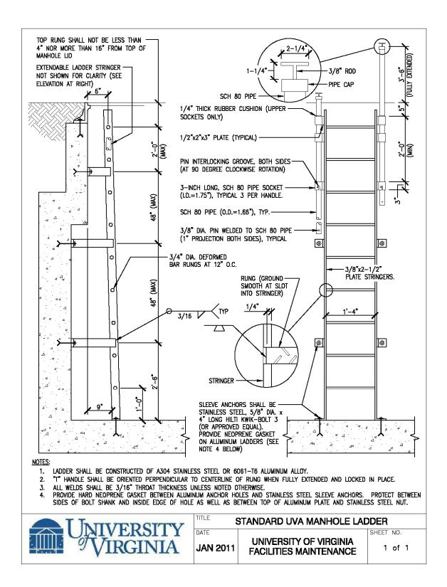
Figure 13: Standard UVA Vault Ladder for Steam Tunnels and Manholes Greater than 10' Deep [not required for Electrical manholes]
