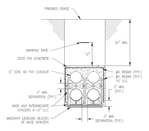
**Figure 15: Electrical Ductbank Section**
