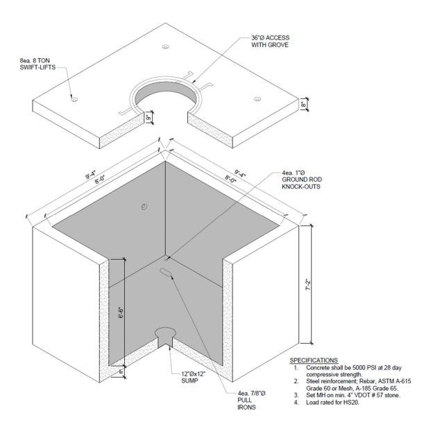
Figure 14: Electrical Manhole/Vault Detail
